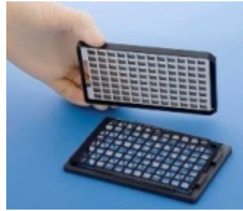
Figure 3b: With a gel-drop microarray printed at the bottom of each well in 96-well plates, 10's of diseases markers can be tested from a single patient sample, 96 patient samples at a time.
